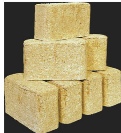
**Figure 8.** Left: A dense forest in Finland. Right: Briquettes from wood chips and sawdust, for energy production
