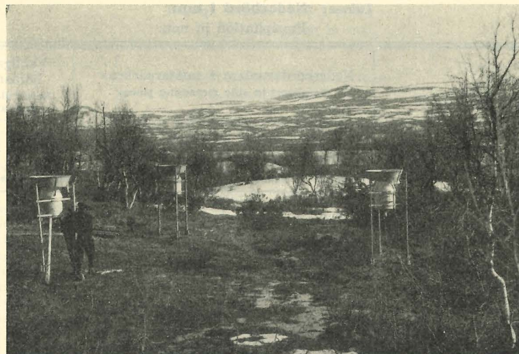
Fig. 8. Nederbördssamlarna i »Mätarparken». Fot. maj 1933. The totalizers in »the measuring place». Of the three totalizers one has a big, one a small and the third no slit between the cylindrical and conical part of the gauge.
