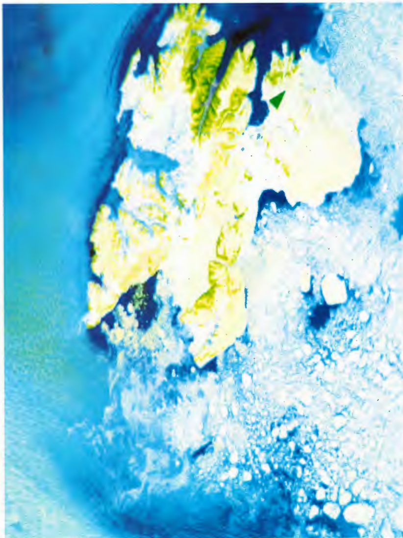
Figure 6: RGB image from AVHRR from 870527. The image demonstrates the veering of the westerly wind to the north when reaching Spitsbergen.
