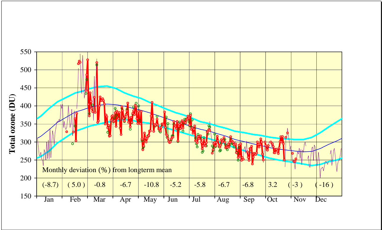
Figure 6 Daily 'noon' values of total ozone recorded by Brewer #006 (red) and by Dobson #30 (green) at Vindeln in 2002. Long-term mean and standard deviation are from Uppsala 1951-1966. The values at the bottom are the monthly deviations (percent) from the long term monthly means. All data refer to bass-Paur scale. Missing data are replaced by TOMS V6 data (thin line).
