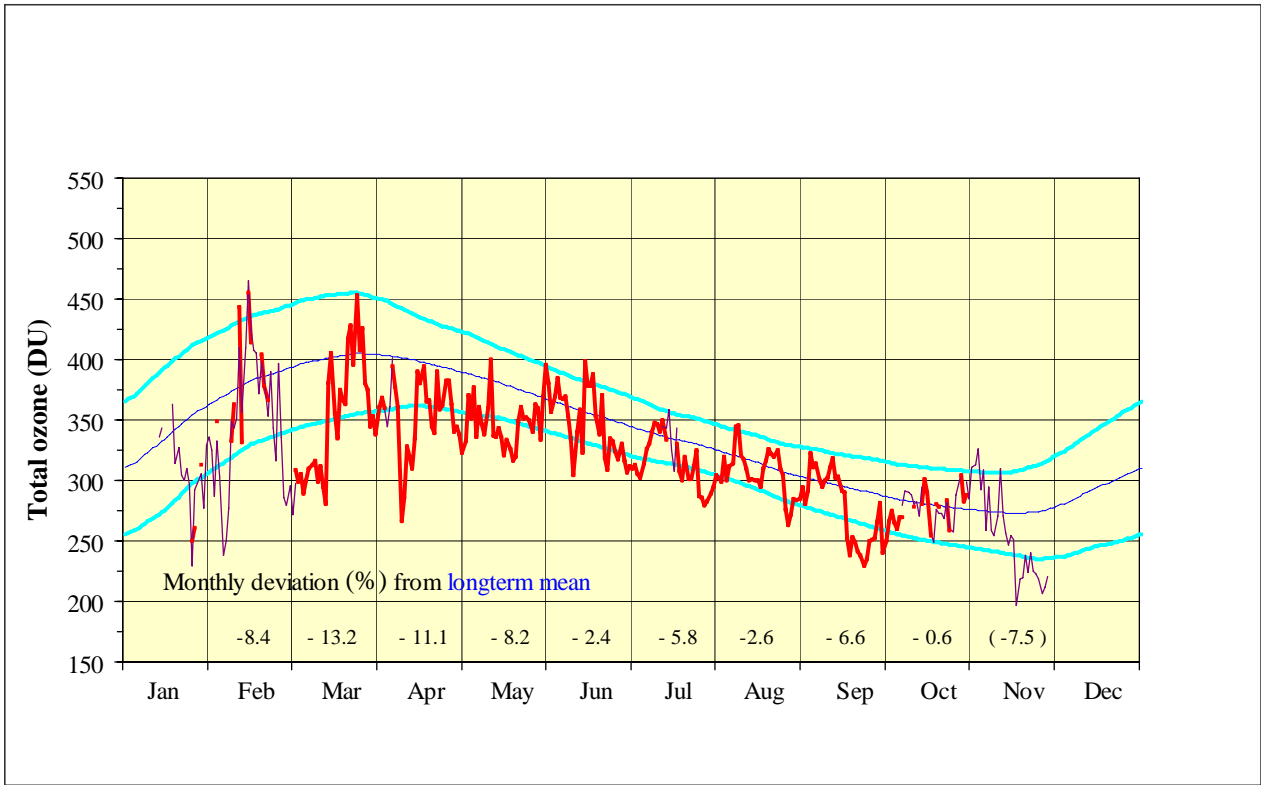
Figure 4 Daily 'noon' values of total ozone recorded by Brewer #006 (red) and by Dobson #30 (green) at Vindeln in 2000. Long-term mean and standard deviation are from Uppsala 1951-1966. The values at the bottom are the monthly deviations (percent) from the long term monthly means. All data refer to bass-Paur scale. Missing data are replaced by TOMS V6 data (thin line).
