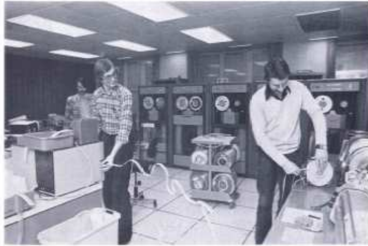
Figure 5: Operators in action with the SMHI D21 computer, input of paper tapes with observation data
