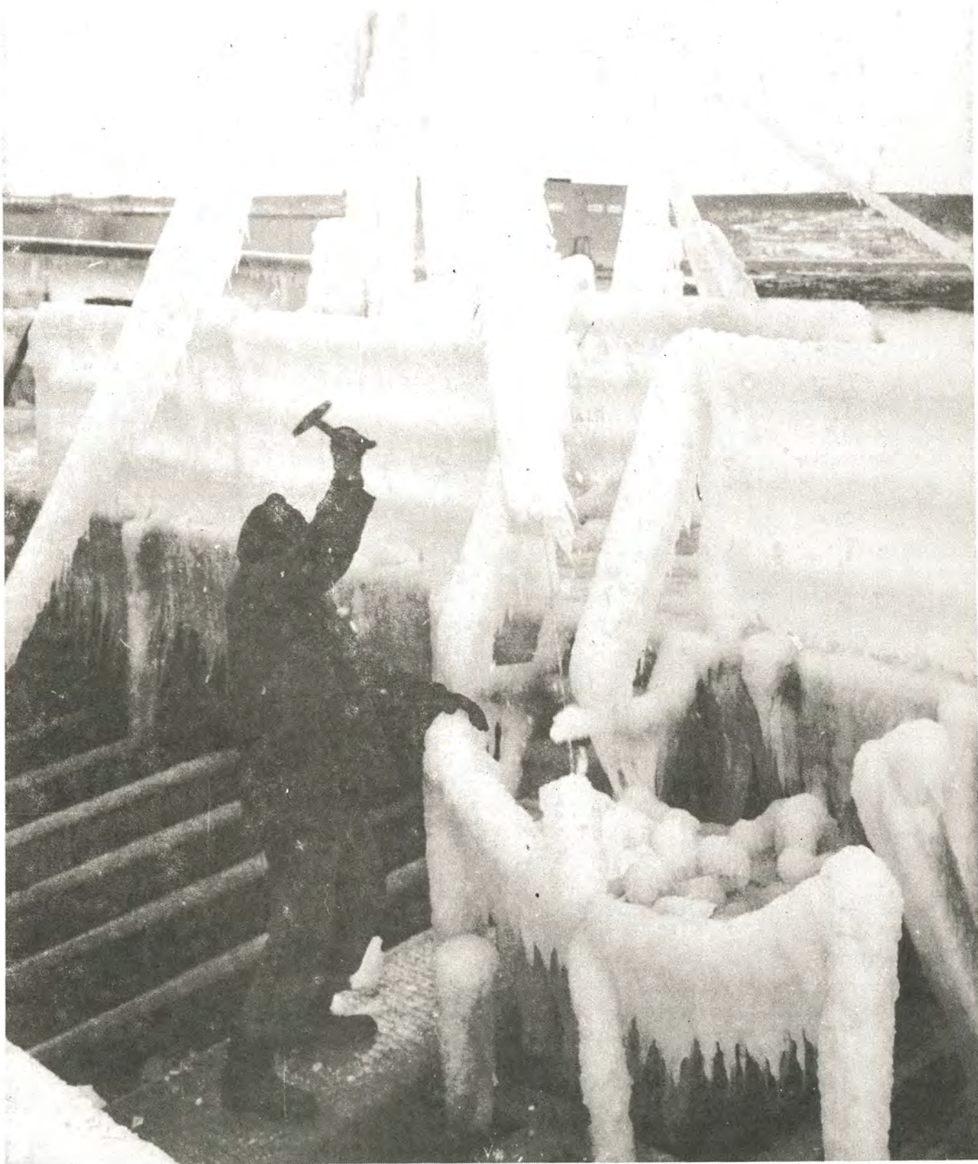
Figure 17. m/s Alchemist Kiel, 9/12 1971. One very usual method for removal of icing is demonstrated.
