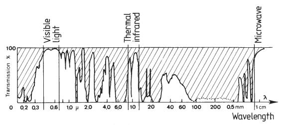
Figure 3 - The electromagnetic spectrum
