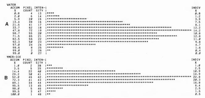
Figure 26- Histogram showing the intensity distribution of areas with water (a.) and with sea ice (b.)
