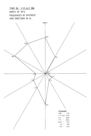
Figure 10 - Frequencies of different wind directions and wind speeds for the period 5 - 31 July 1980 (north of 780N)
