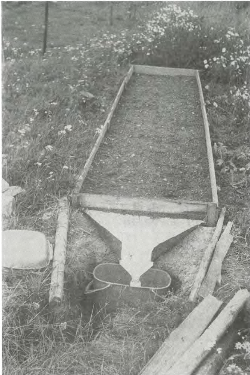
Figure 2. Photo of the plot construction (the plot without vegetation). The plate and the small catching container were normally covered by a plastic roof. The mean slope of the plot is about 5^\circ on a medium clayey soil.
