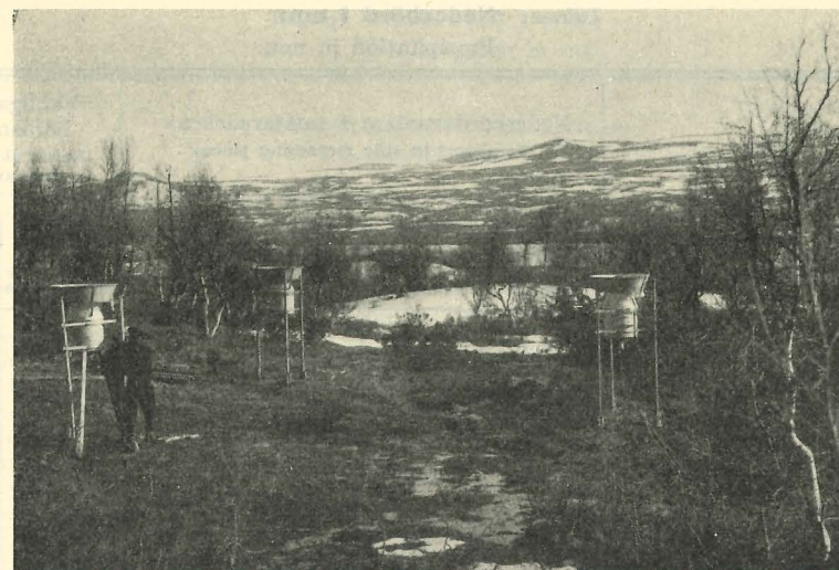
Fig. 8. Nederbördssamlarna i »Mätarparken». Fot. maj 1933. The totalizers in »the measuring places». Of the three totalizers one has a big, one a small and the third no slit between the cylindrical and conical part of the gauge.
