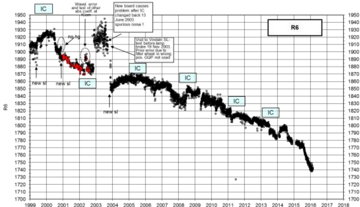
Figure 4.4. Standard lamp test value R6 for Brewer #6 over the period 1999-2015. Comparisons (IC) and lamp changes are noted as well as comments to some outliers.
