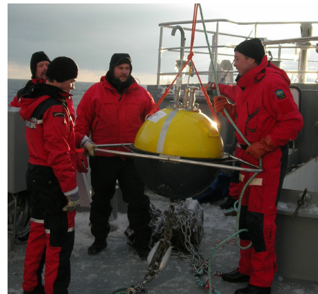
Figure 32. One of SMHI:s buoys for wave measurements. Also sea water temperature is recorded. Data are presented in near real time at www.smhi.se
