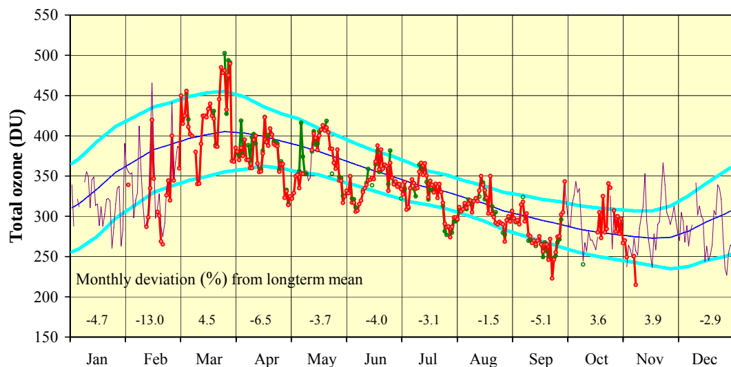
Figure 5.6 Daily 'noon' values of total ozone recorded by Brewer #006 (red) and by Dobson #30 (green) at Vindeln in 2008. Long-term mean and standard deviation are from Uppsala 1951-1966. The values at the bottom are the monthly deviations (percent) from the long term monthly means. All data refer to Bass-Paur scale. Missing data are replaced by satellite data (purple line).
