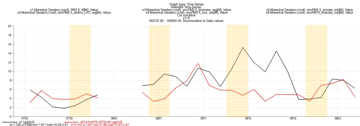
Fig. 4.4.12 Monitored and simulated daily \text{PM}_{2.5} levels at Marechal Deodoro roof level: Monitored (black), simulated (red) consisting of regional model contributions from anthropogenic and biomass burning plus local impact of buses, private vehicles and industry within the Curitiba municipality. The local contribution was modified according to the results obtained from the street canyon Marechal Deodoro.
