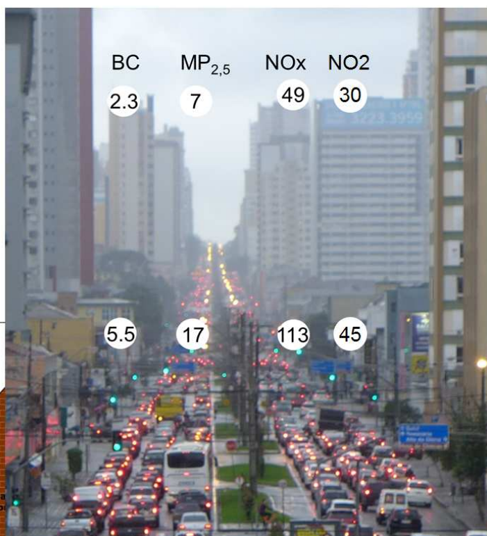
Figure 4.5.6 Overview of how local traffic can increase air pollution levels inside a street canyon in Curitiba, adding to the urban background levels registered at roof level. Measurements made in the Marechal Deodoro street canyon. Note: The photo is from another street, used for illustrating how the buildings contribute to a canyon-like structure with reduced ventilation (also illustrated in the figure to the left).
