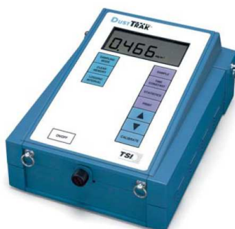
Figure 3.3.4 DustTrak device used for \text{PM}_{2.5} continuous measurement.
