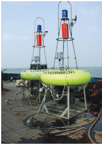
Figure 33. The SmartBuoys are operated by CEFAS in the waters surrounding the United Kingdom (map to the right). Several sensors and a water sampling device is found at c. 1 m depth. CEFAS is the Centre for Environment, Fisheries & Aquaculture Science a UK government agency.
