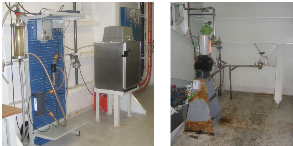
Figure 28. The FerryBox system on Finnmaid. the ship that operates the route Helsinki-Lübeck. Left: De-bubbler, sensors and water sampling system. Right: water inlet and pump.
