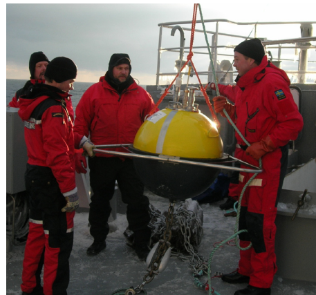
Figure 32. One of SMHI:s buoys for wave measurements. Also sea water temperature is recorded. Data are presented in near real time at www.smhi.se
