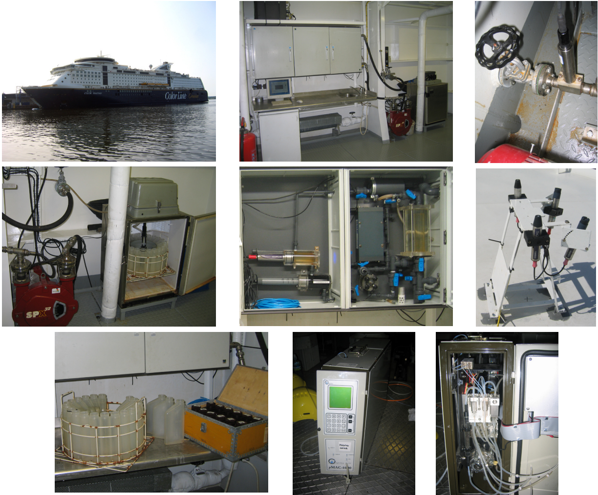
Figure 27. FerryBox system on Color Fantasy. the ship that operates the route Oslo-Kiel. From left to right, top row: ship, below deck system and water temperature sensor at water inlet. Middle row: Pump and refrigerated water sampling system, flow through system and sensors and irradiation sensors on deck. Bottom row: water samples and automated nutrient analyser (to be included in 2009).
