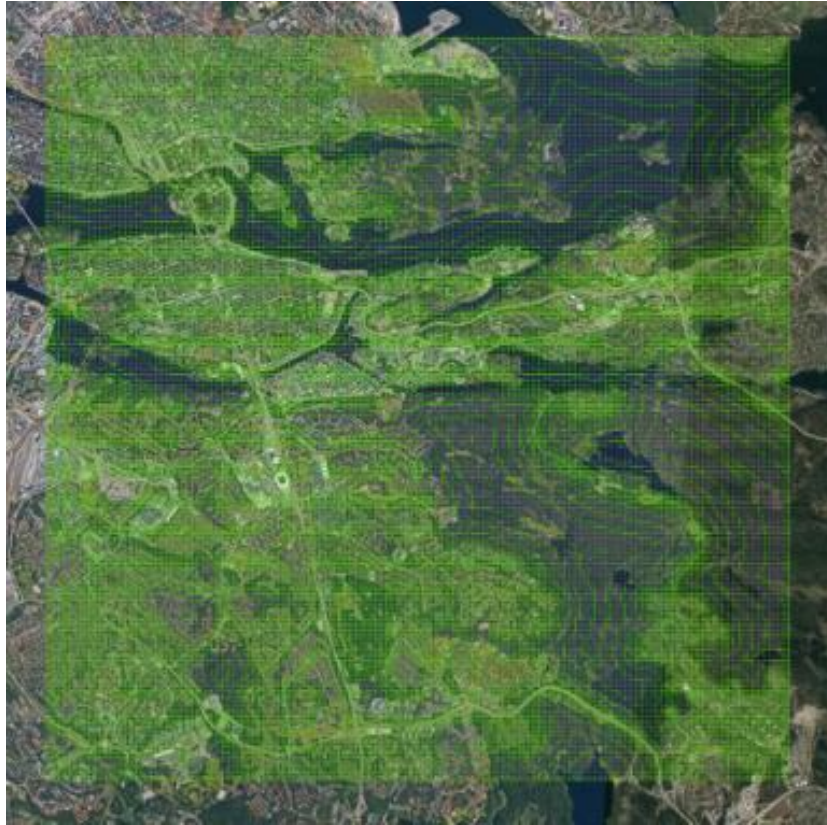
Figure 10. An example of a refined grid. Close to emission sources receptor points are dense, and further away from the sources there are fewer and fewer receptor points.
