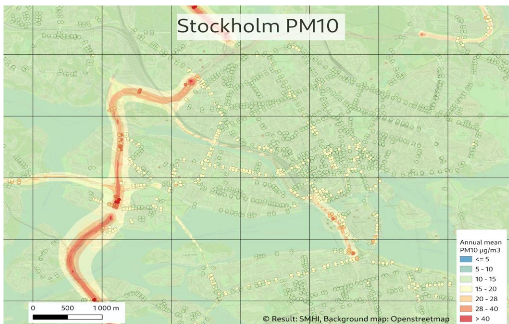
Figure 15. Annual PM10 concentrations over Stockholm 2019. Circles represent the total concentration from regional, urban and street canyon contributions. Fields represent background concentrations from regional and urban contributions. The concentration intervals in the legend are grouped according to annual threshold values. They are; the annual air quality standard (40), upper and lower assessment thresholds (28 and 20), WHO annual guideline (20), and the Swedish air quality objective (15). Concentration unit: \mu\text{g}/\text{m}^3 .
