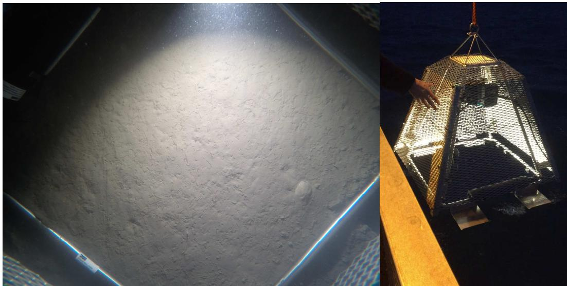
Figure 1. The drop-video rig is equipped with head lights and two Go-pro cameras that both takes pictures and films the bottom. The image is taken at the station P2 in Skagerrak.
