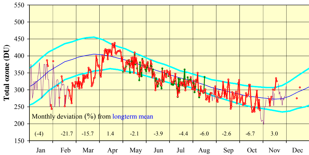
Figure 5.6 Daily 'noon' values of total ozone recorded by Brewer #006 (red) and by Dobson #30 (green) at Vindeln in 2005. Long-term mean and standard deviation are from Uppsala 1951-1966. The values at the bottom are the monthly deviations (percent) from the long term monthly means. All data refer to Bass-Paur scale. Missing data are replaced by satellite data (purple line).
