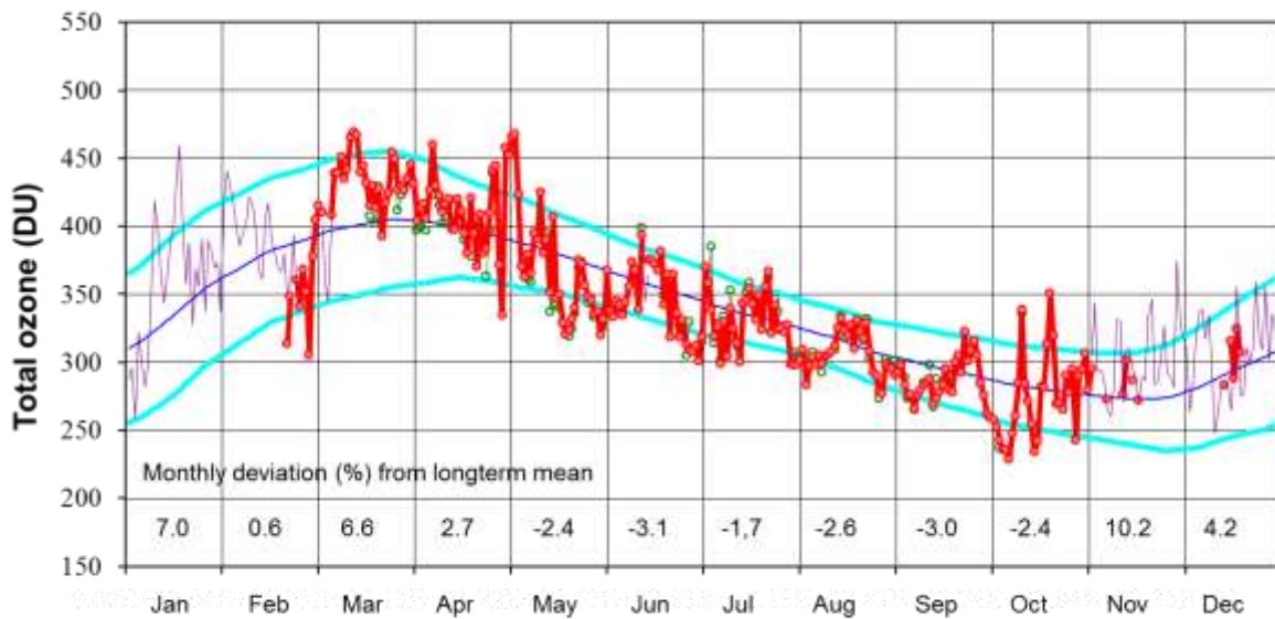
Figure 5.6 Daily 'noon' values of total ozone recorded by Brewer #6 (red) and by Dobson #30 (green) at Vindeln in 2013. Long-term mean and standard deviation are from Uppsala 1951-1966. The values at the bottom are the monthly deviations (percent) from the long term monthly means. All data refer to Bass-Paur scale. Missing data are replaced by satellite data (purple line).
