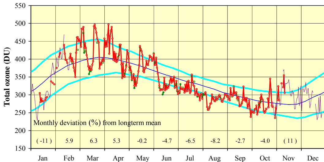
Figure 5.4 Daily 'noon' values of total ozone recorded by Brewer #006 (red) and by Dobson #30 (green) at Vindeln in 2006. Long-term mean and standard deviation are from Uppsala 1951-1966. The values at the bottom are the monthly deviations (percent) from the long term monthly means. All data refer to bass-Paur scale. Missing data are replaced by satellite data (purple line).
